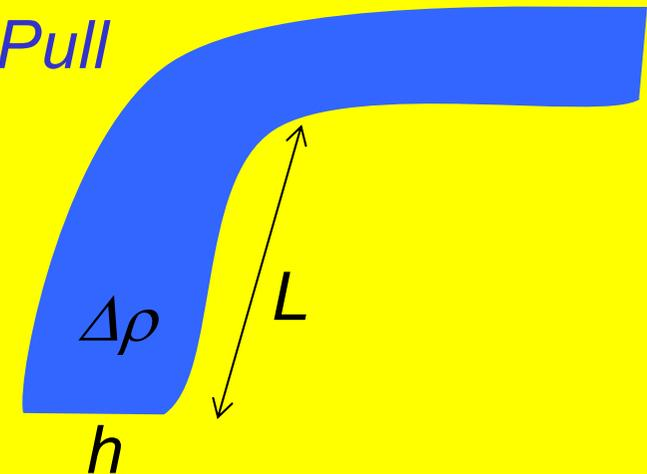
$$F_{SP} = \text{Excess weight of slab} = \Delta\rho ghL$$
